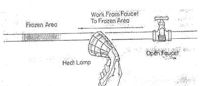
How do you know your pipe is frozen? After a bitterly cold night, you turn on your tap and instead of a steady gush of water you get a sickly trickle followed by...nothing. Since water expands when it freezes -- and pipes don't -- a frozen pipe is in danger of bursting. It needs to be thawed.
